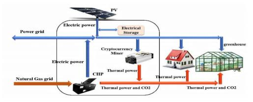
Fig. 1. Proposed Energy Hub Structure
