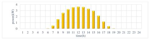
Fig. 3. Power generated by PV during the day
