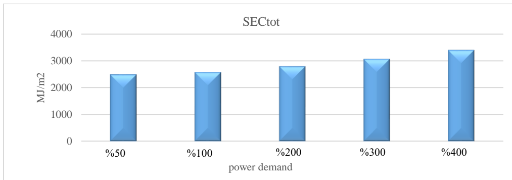
Fig. 8. Changes of SEC tot with the demand changes (for the proposed structure)
