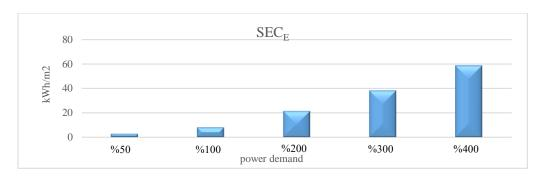
Fig. 7. Changes of SECE with the demand changes (for the proposed structure)
